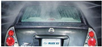
The same contour-following touch-free cleaning system found on Mark VII's AquaJet XT 700, which utilizes 28 zero degree turbo nozzles with built-in rocker rocker panel blasters, accommodates customers who prefer a touchless wash.
