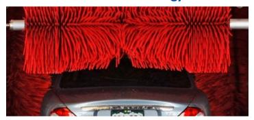
→ Our patented SofTecs® foam material gently and safely cleans and polishes vehicles while minimizing the electricity, water and chemicals consumed when customers choose a soft-touch wash.
