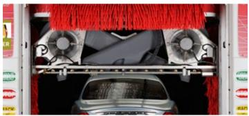
→ Tracks vehicle from the optimal distance to minimize energy consumption while avoiding obstacles such as antennas and roof racks. AquaDri® static on-board and freestanding dryers are also available for the ChoiceWash XT.
