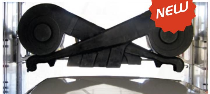
→ Tracks vehicle from the optimal distance to minimize energy consumption while avoiding obstacles such as antennas and roof racks. AquaDri® static on-board and freestanding dryers are also available for the SoftWash XT.
