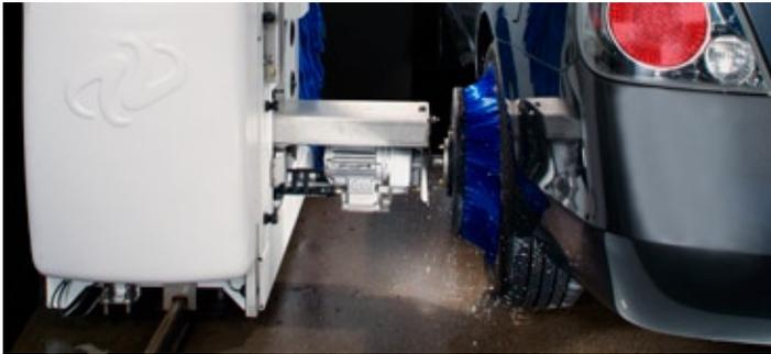
→ Resolves the number one complaint from consumers: dirty wheels. Wheel brushes with integrated rim spraying rotate both directions to clean convoluted wheel surfaces and allow the operator to charge more for the premium wash package.
